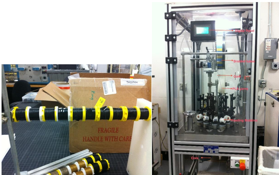
(a) Ten 2-0 PP black monofilament sutures wound on small bobbins ready to provide a central core. (b) 16 spindle Steeger braiding machine
