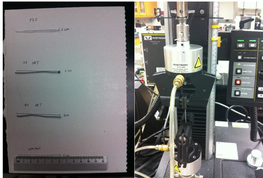
(a) 60 mm long nerve guide specimens for tensile strength testing
