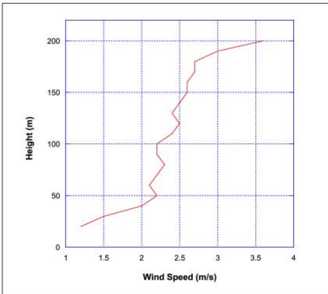
Figure 4.9a Model 4000 miniSODAR vertical wind profile (m/s) over lower Manhattan valid 05 UTC (00 LT) 31 January 2002. The near surface wind direction was from the east-southeast.
