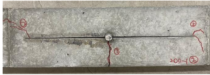
Figure 14. Test specimen with crack for imaging
