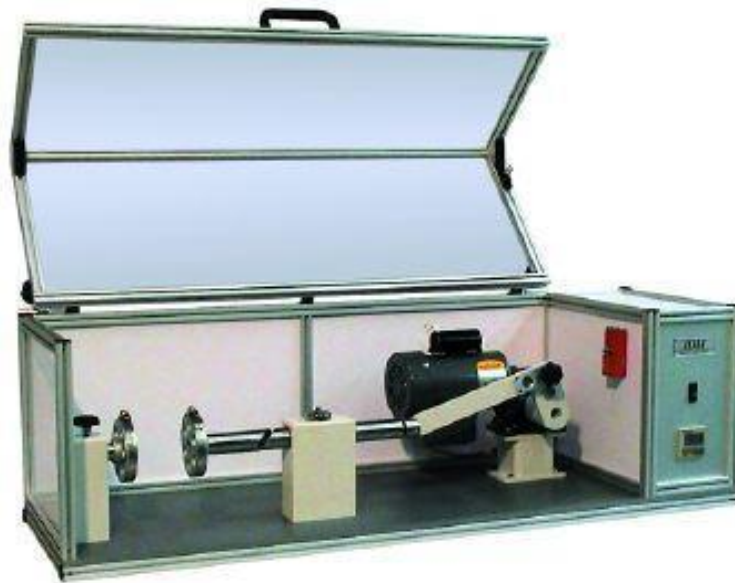
Figure 5.4 Gelbo Flex Tester for evaluating the Flex durability of nanofiber mats deposited on fabric substrate.
