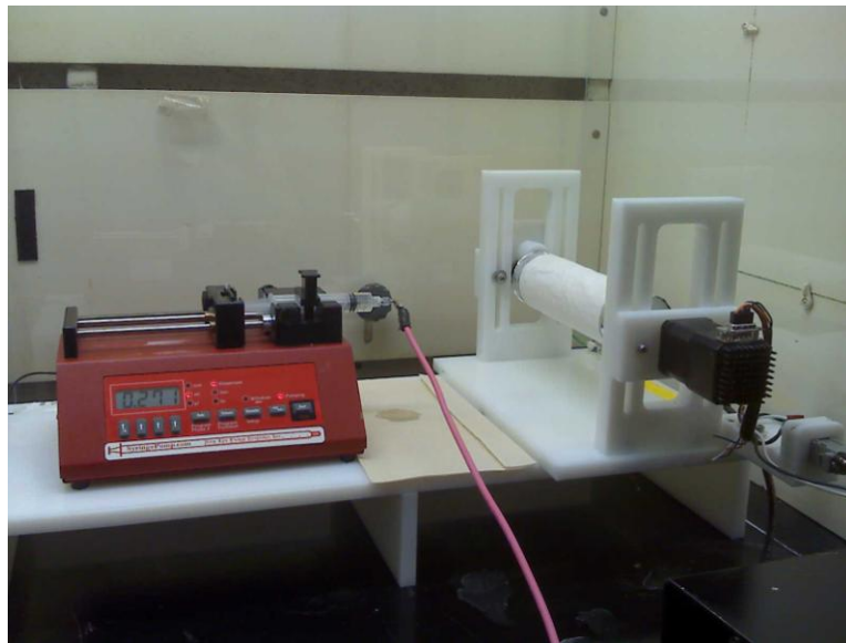
Figure 3.1 Photograph of electrospinning setup.
