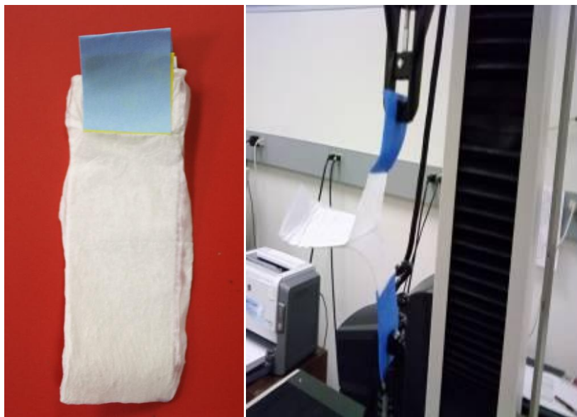
Figure 6.3 Adhesion strength measurement between nanofiber mat and fabric; a) Nanofiber mat and fabric with short tape attached b) sample held in Instron instrument grips.
