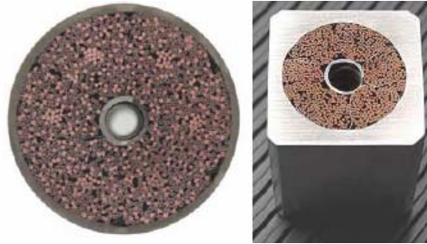
Figure 13. The typical cable crosssection for TF coils (left) and CS / PF coils (right).
