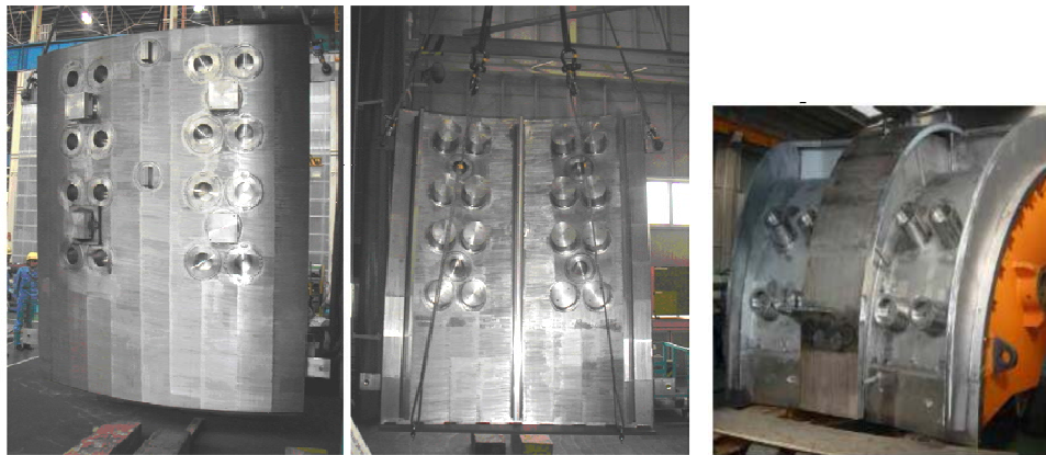
Figure 7. Partial mockups of the VV sector.
