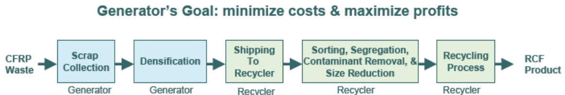
Figure 1.25 Waste Generator Model. The scrap generator profits, while the recycler takes a hit giving an overall value of zero. [62]
