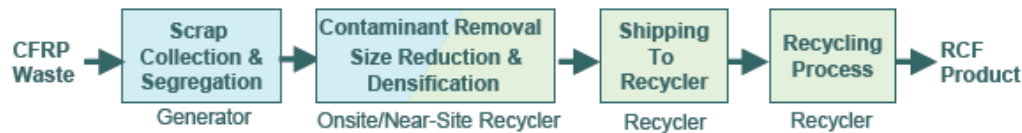
Figure 1.27 Cooperative Model. Both waste generator and recycler bear the burden of preparing the scrap but both are able to profit since the carbon fiber recovered is highly valuable.[62]
