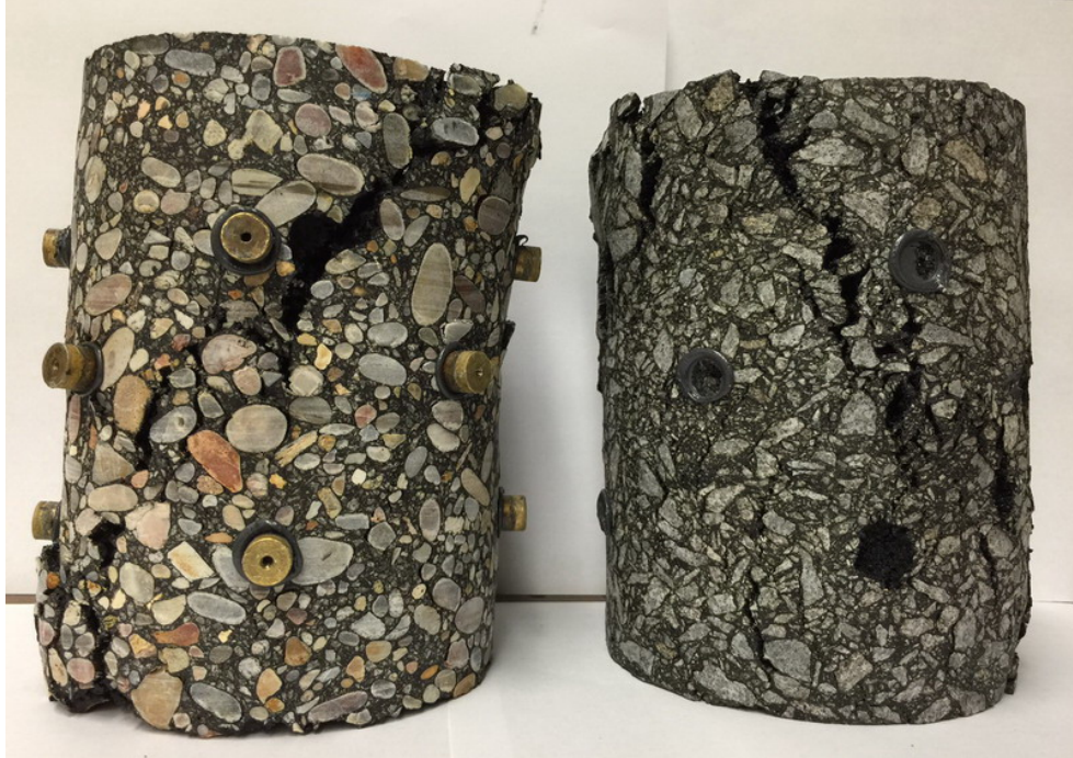
Figure 6-19 Specimens fractured after the monotonic compression tests.
