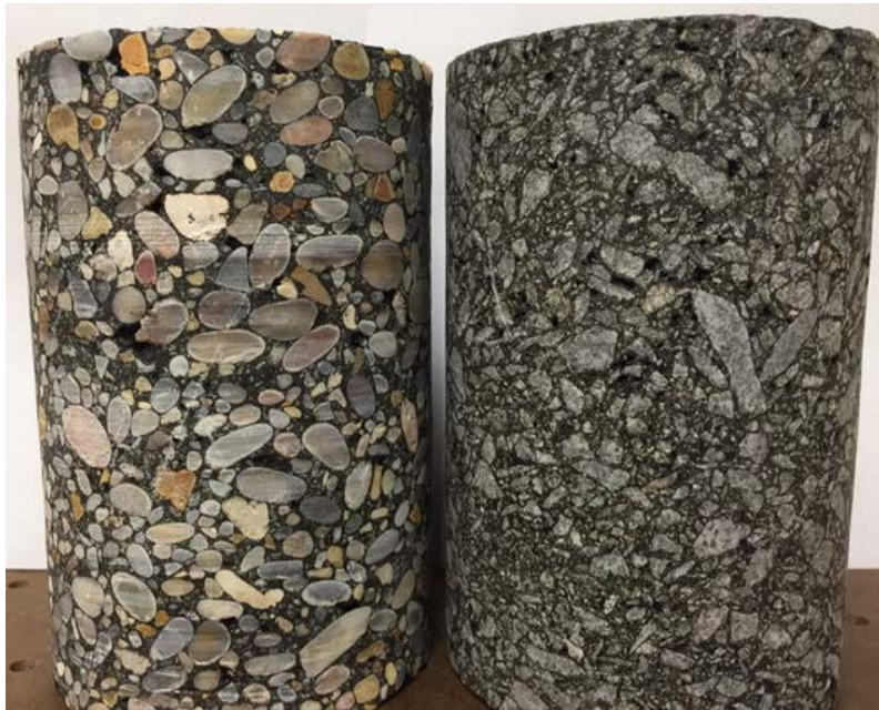
Figure 6-16 Test specimens for the River Gravel mix (left) and FHWA ALF mix (right).
