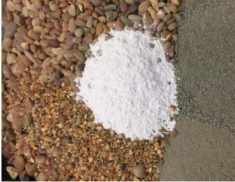
Figure 6-15 One batch of the total aggregate (including lime) for half a specimen.
