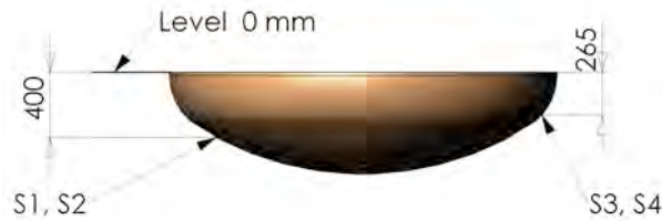
Figure 4. Strain gauge locations in PPOOLEX
