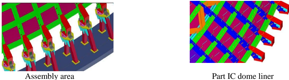
Figure 2. Seating arrangement in the assembly area and part view IC dome liner seating arrangement
