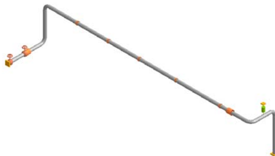
Figure 2: Layout of TDFP steam supply piping
