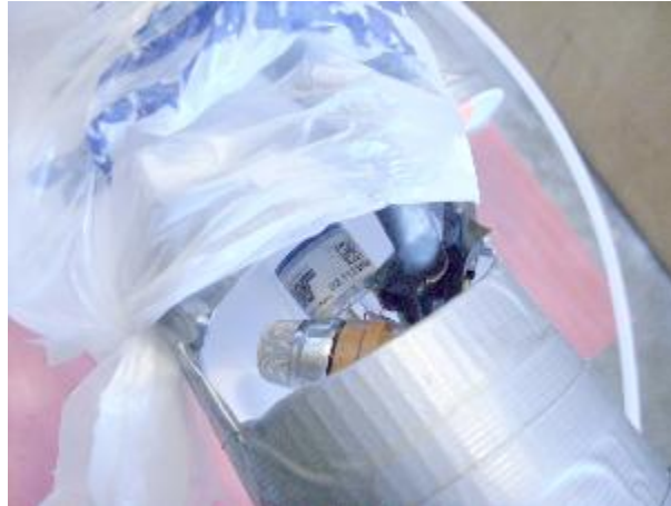
Figure 4.4: Gas Sensors Mounted on the Apparatus
