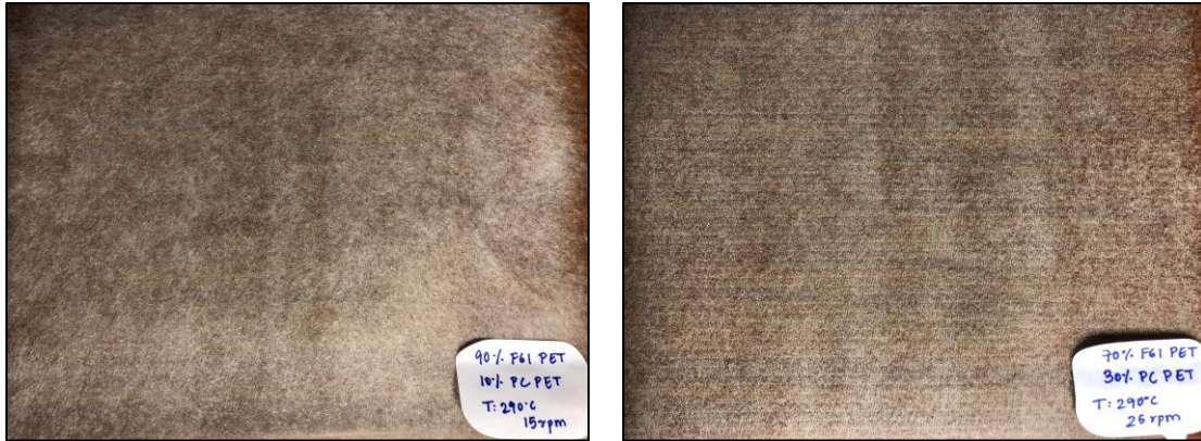
Figure 42. Meltblown webs of virgin PET: Rec PET grade 2 in 90:10 ratio (left) and 70:30 ratio (right).
