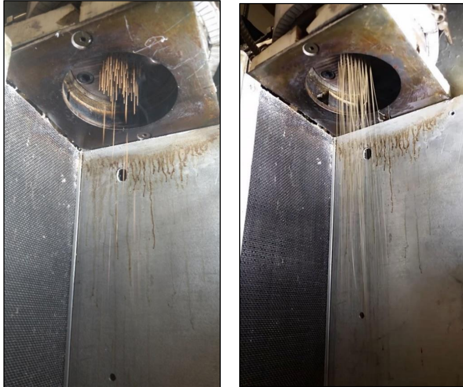
Figure 34. Rec PET grade 1 (left) and grade 2 in free fall (right) on Homocomponent Line (Hills system).
