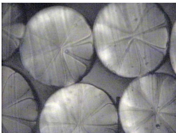
FIGURE 5.1, Fiber Cross section at 0.5 gram per hole per minute throughput rate
