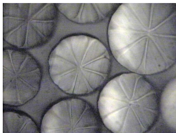
FIGURE 5.2, Fiber Cross section at 0.7 gram per hole per minute throughput rate
