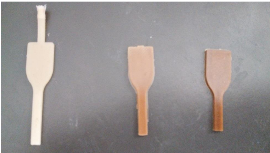
Figure 3. (Left to right): 30 weight percent HW LDPE based WPC, 30 weight percent HW PP based WPC and 50 weight percent HW PP based WPC.
