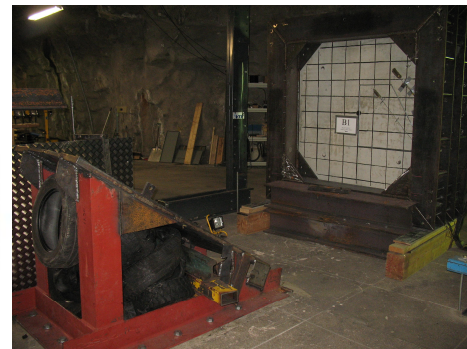
Figure 1. Left: Test apparatus. Right: The wall in the test B1 as mounted on the frame.
