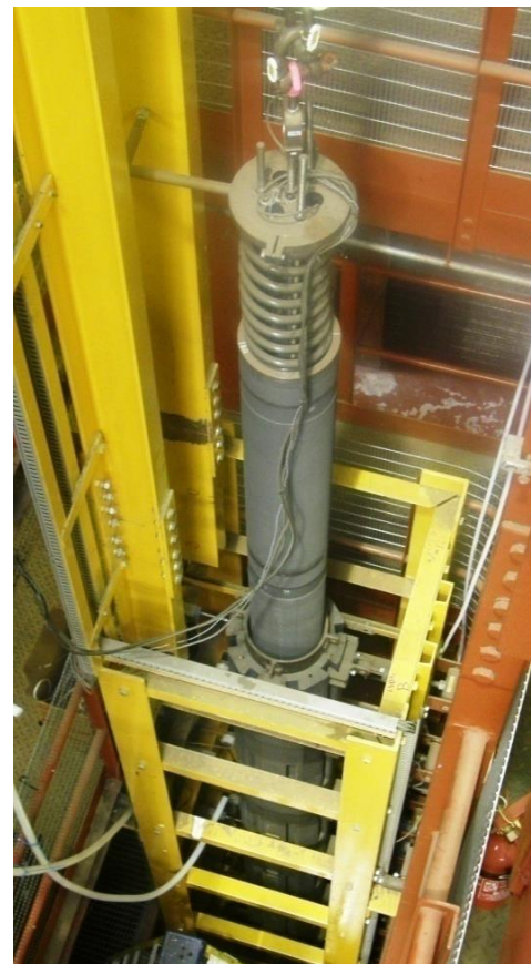
Figure 5. Replica fuel stringer, partially inserted into a fuel channel rig
