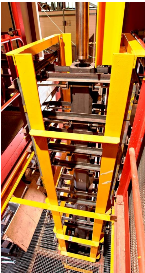
Figure 4. Replica control rod (top) before being lowered into a control channel rig
