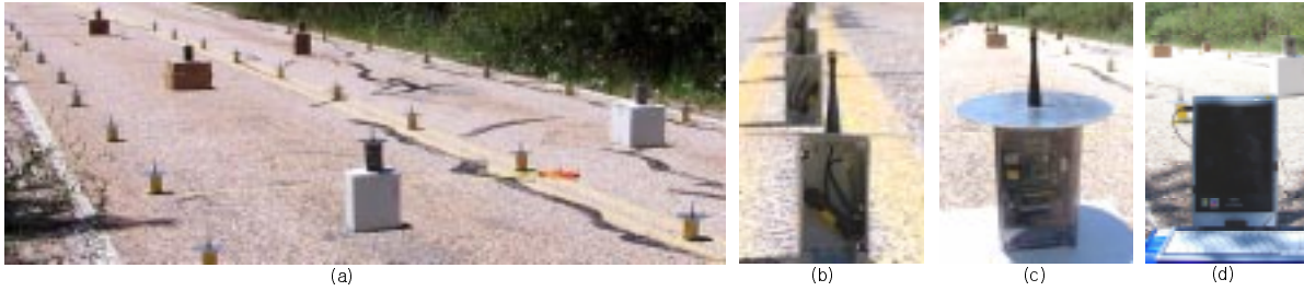
Figure 6.3: Pictures from the field deployment: (a) overall network, (b) Mica2 motes, (c) Stargate monitor, and (d) tablet PC for data collection.
