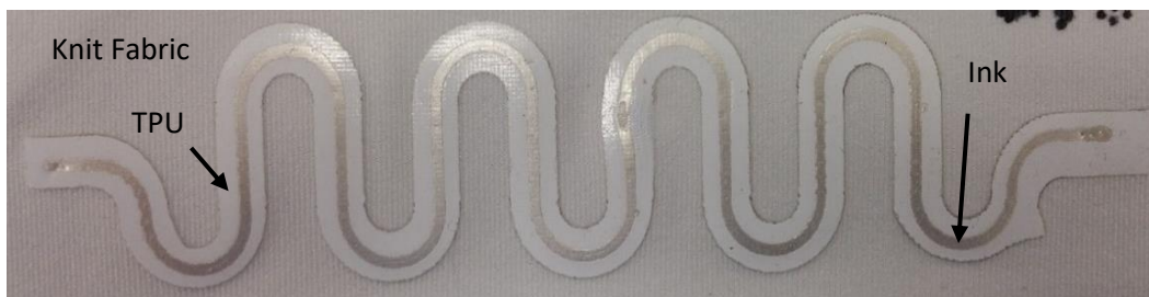
Figure 2- 7 Ag/AgCl screen printed interconnect on TPU substrate, heat pressed on knit fabric [62]. Picture credit: NEXT (nano-extended textiles) research group.
