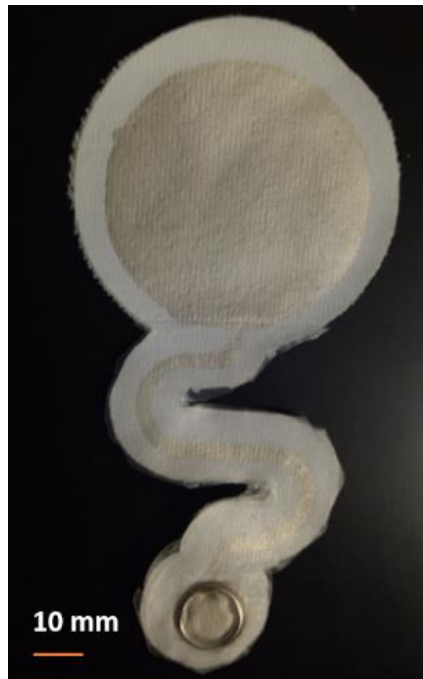
Figure 5- 2 An electrode used for the infant onesie. It is Ag/AgCl ink screen-printed on white TPU film and a snap is the output at the end of the interconnect.
