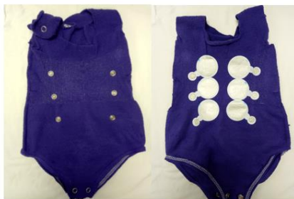
③ Onesie with elastic inlay and 6 electrodes on the front to test different placement
