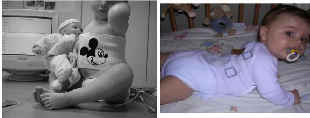
Figure 2- 2 Left: Prototype belt with textile electrodes integrated into the mickey mouse ears[33]. Right: Prototype baby pajama with sensors and circuits, worn by a 21-week-old baby[34].
