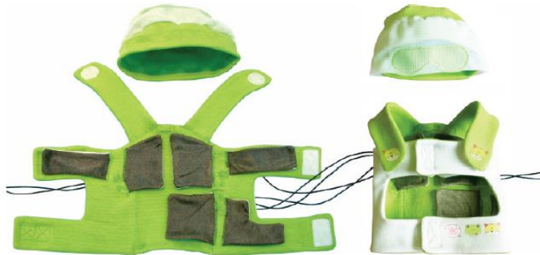
Figure 2- 1 Prototype of the Smart jacket with textile sensors for ECG monitoring[32]
