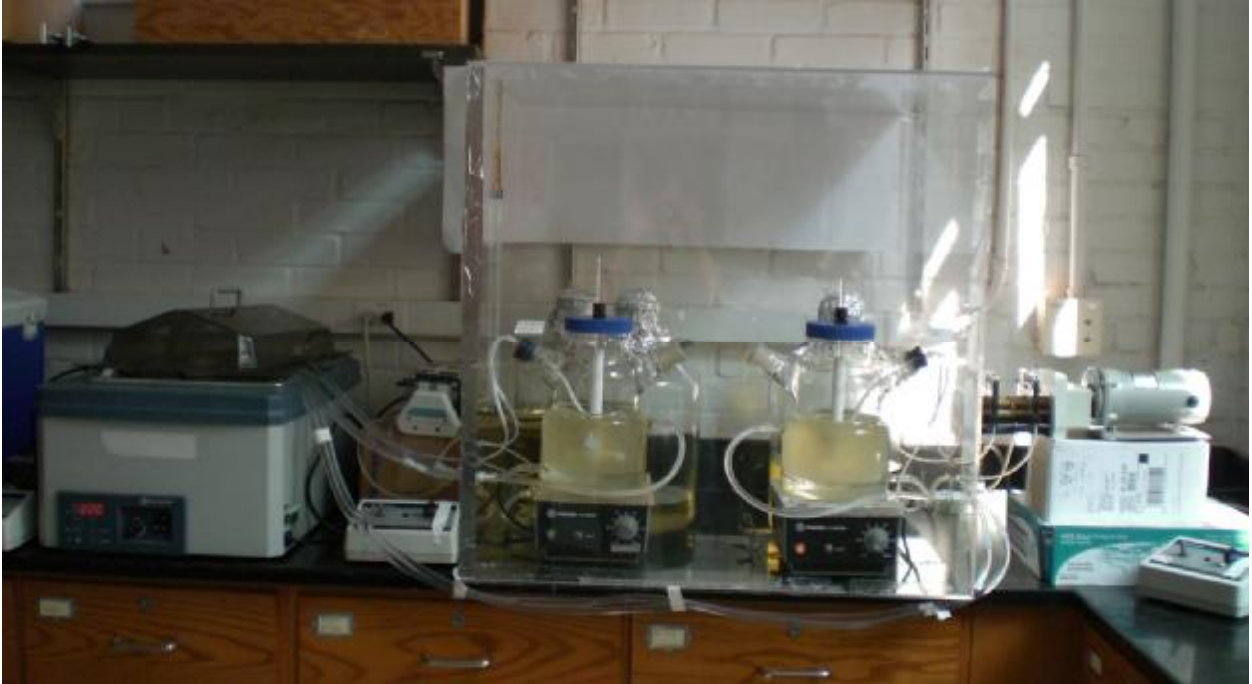
Figure 3.2 - Overall setup of chemostat reactors From L to R: cooler, water bath, pump and controller 1, Plexiglas box containing chemostat/feed/effluent systems 1&2, pump and controller 2.
