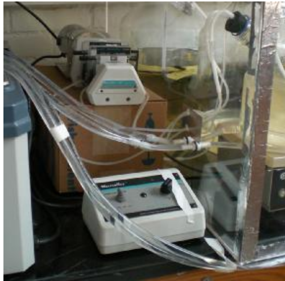
Figure 3.3 - Close-up of pump (to show fine and coarse adjustments)
