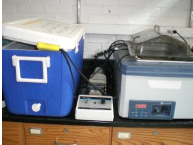
Figure 3.4 - Cooler and water bath setup
