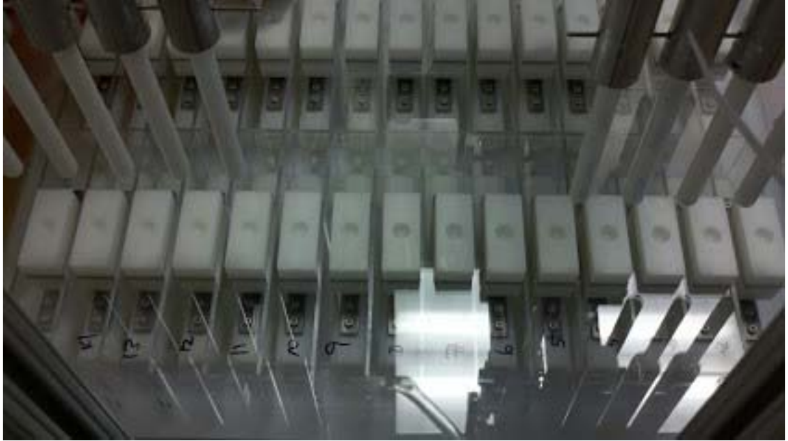
Figure 4-9 Top view of upper tank of test rig. Note the loading blocks with hemi-sphere machined in top and the acrylic aligning the loading blocks (numbers are written on acrylic to denote chamber position, not sample identification)
