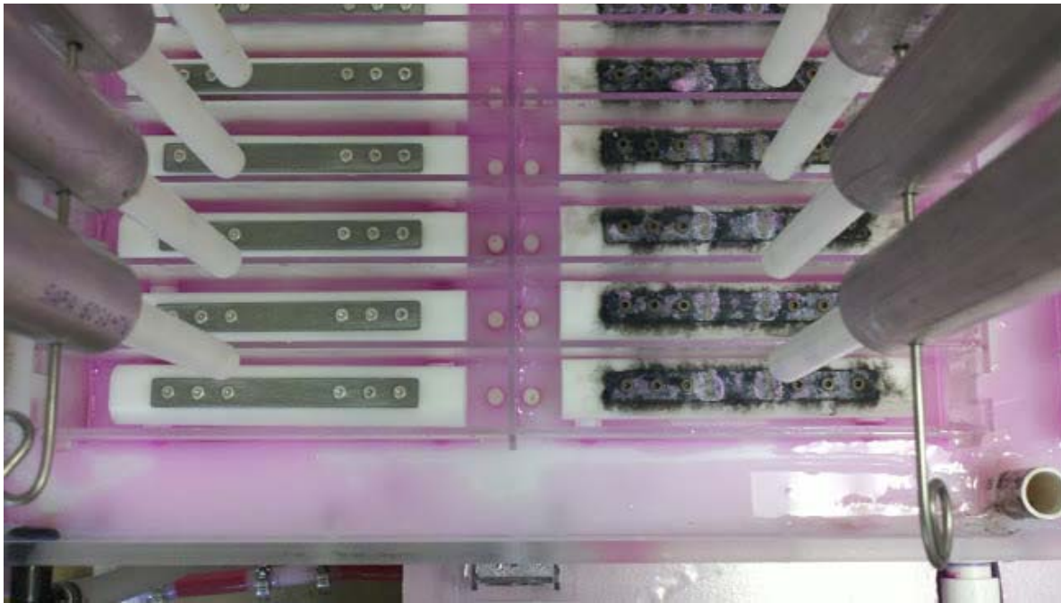
Figure 4-11 Testing apparatus view from above showing individual testing locations, orificed drains (center) and makeup water inlets at the sides. Note the corrosion on the samples to the right (after 2 weeks) as compared to the newly inserted 8-week samples
