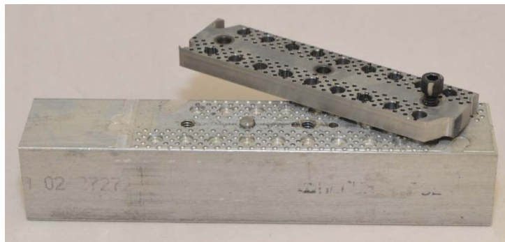
Figure 3-3 Machining fixture in open position showing aligning pins
