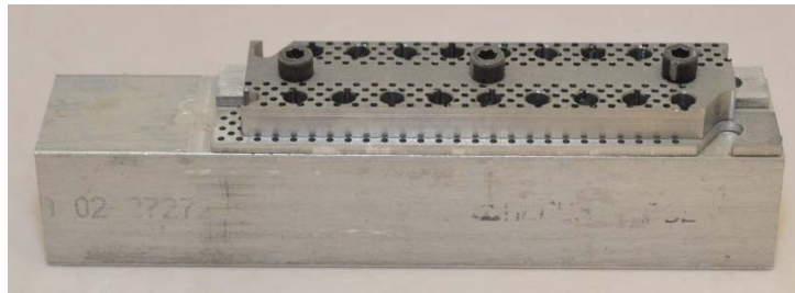
Figure 3-2 Machining fixture in clamped position
