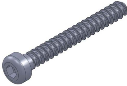
Figure 4-2 Bone screw model based on a 3.5 mm cortical bone screw
