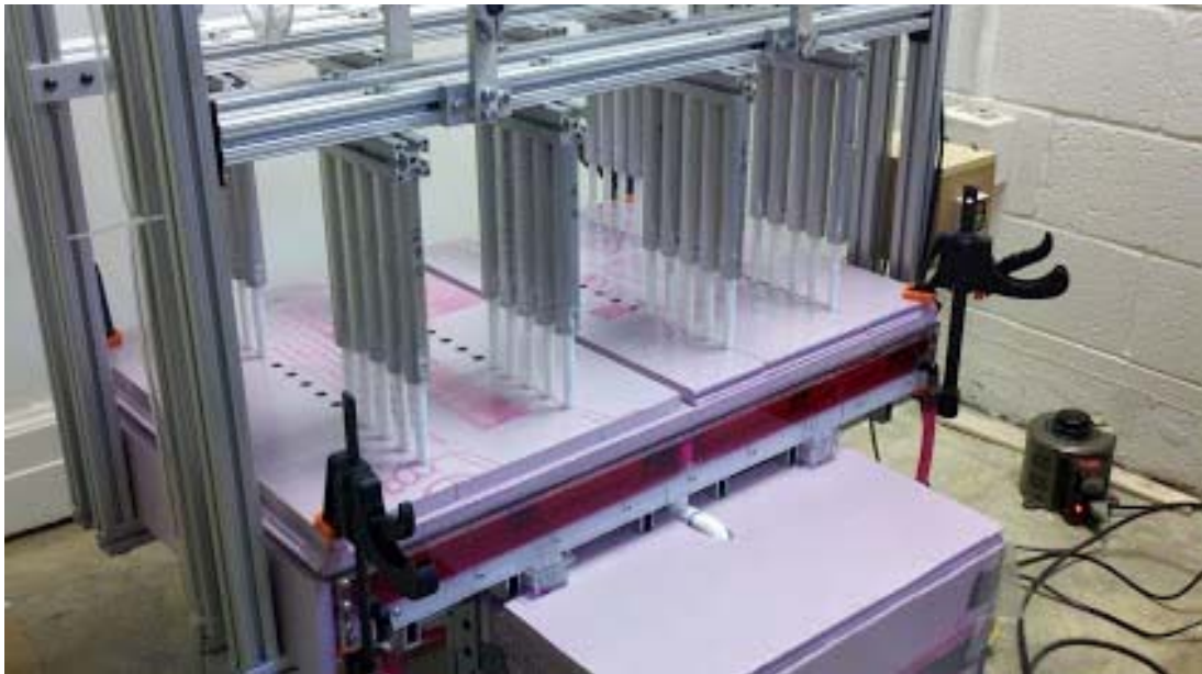
Figure 4-10 Assembled and operating testing rig. Note: dynamic loading is in the foreground, static loading in the background and no-load samples were in the middle
