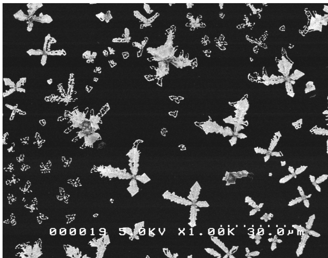
Figure 4-4: Scanning electron microscopy image of 250 mg/L fullerol in 0.9% saline solution (1,400x magnification).
