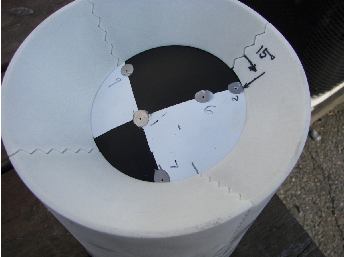
Figure 3.9: PTM inside sabot at non-zero angle of attack and sideslip
