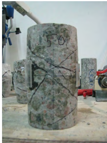
Figure 1: Specimens after tri-axial tests with confinement of 47 MPa and 100 MPa
