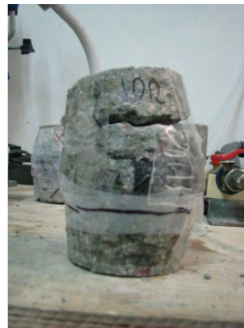
Figure 1: Specimens after tri-axial tests with confinement of 47 MPa and 100 MPa
