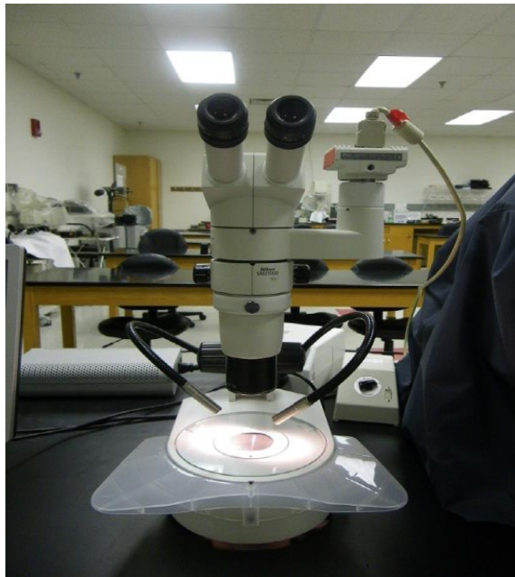
Figure 28: The Nikon stereoscope used to visualize the samples for the microscopic analysis [15].
