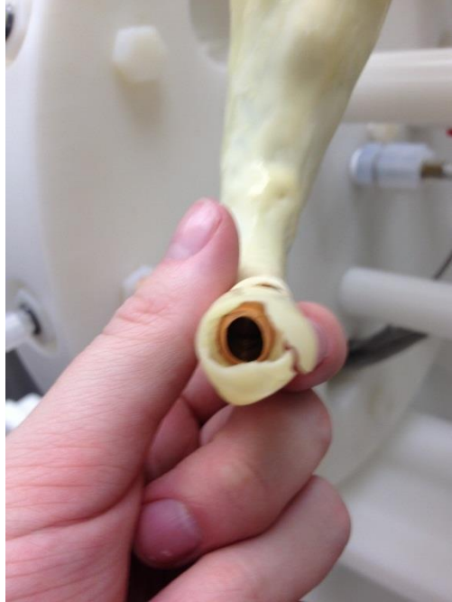
Figure 27: The piece of copper tube inserted to allow silicone tape to be bound around the tear without occluding the limb.
