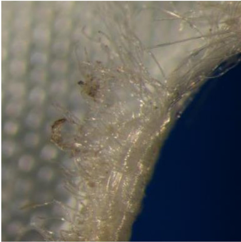
Figure 37: Evidence of fraying at the edge of the fenestration, as well as some melted and fused fibers. 40x zoom.
