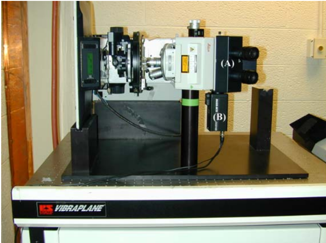
Fig 2.2 A-B Leica Upright Microscope cradled in a sidemount position.
