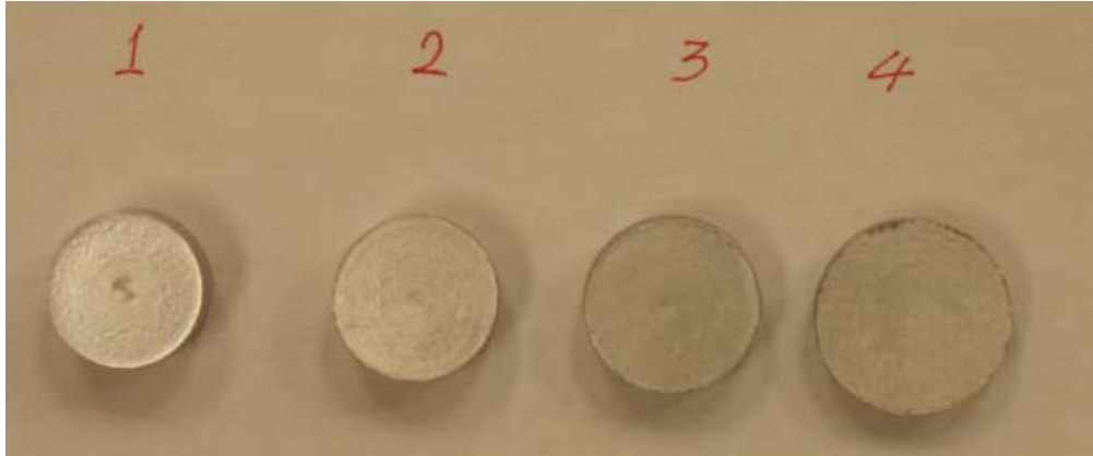
Fig.7- 8 Compressed samples for the flow stress measurement
