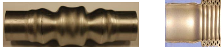
Fig.5- 13 (a) Non-axisymmetric wrinkle (b) Localized wrinkle [16]
