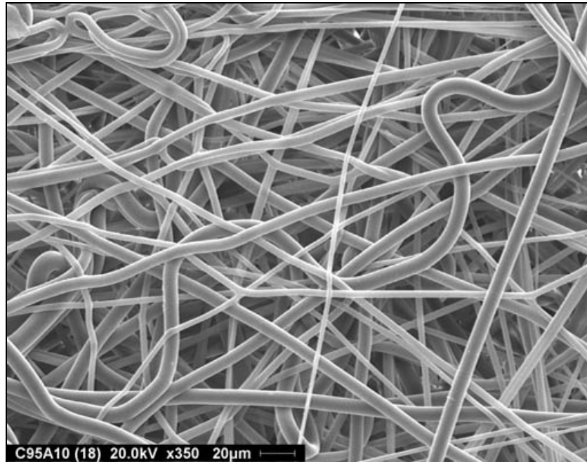
Figure 47: 350X SEM image of S95 melt-blown web at DCD=30.5cm. Courtesy of BASF
