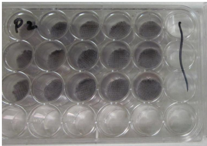
Figure 4.4.4 Cells left on the 3D scaffolds after the MTT assay.
