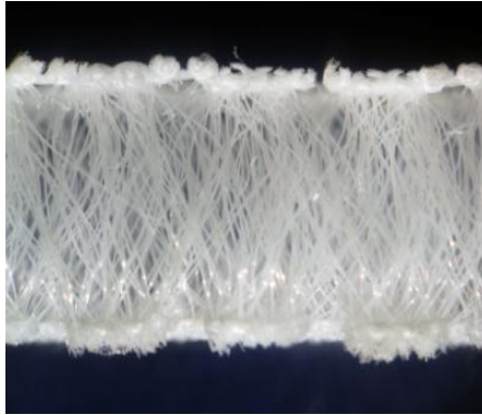
Figure 2.3.4 A spacer fabric knitted from multifilament yarns in the face and back layers and showing criss-crossed monofilament yarns in the middle spacer layer.
