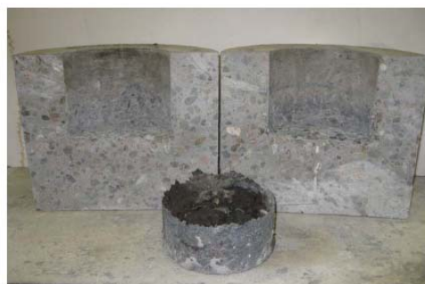
Figure 15: View of spill test specimen C1 after cutting in half
