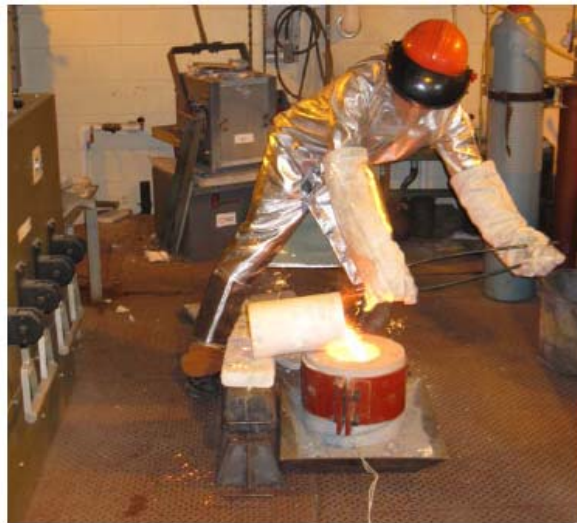
Figure 9: Pouring of molten pig iron from crucible into spill test specimen
