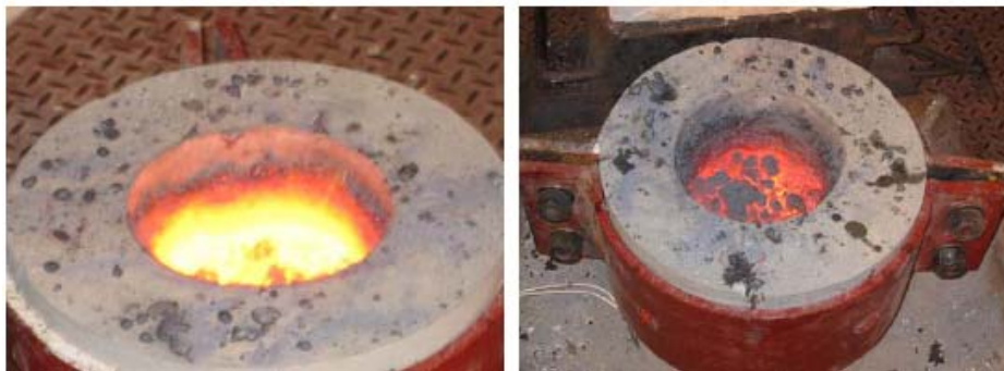
Figure 11: Cooling and hardening of molten pig iron
