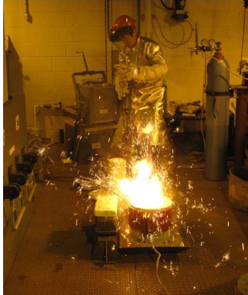
Figure 10: Reaction between molten pig iron and concrete
