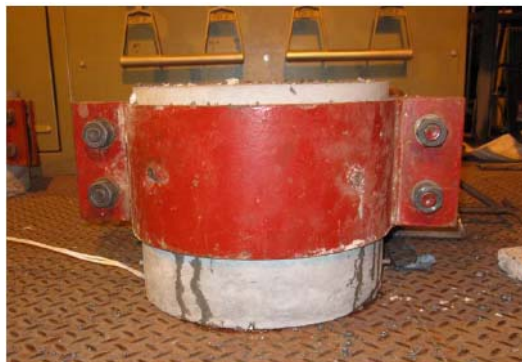
Figure 12: Water seeping out of cracks in spill test specimen
