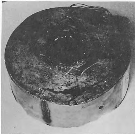
Fig. 6 - SHOCK TEST OF A REINFORCED CONCRETE HOLLOW CYLINDER WITH A WRAPPED STEEL SHEET 0,3 mm THICK
