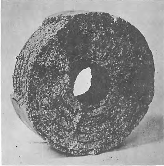
Fig. 3 - DESTRUCTIVE EFFECT ON A REINFORCED CONCRETE HOLLOW CYLINDER
