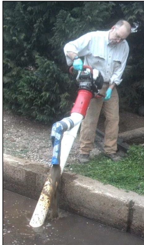
Figure C.3 The Extraction Auger prototype with the 43cc 2 HP engine recycling dairy waste from the settling basin after the addition of the section of reverse flights.
