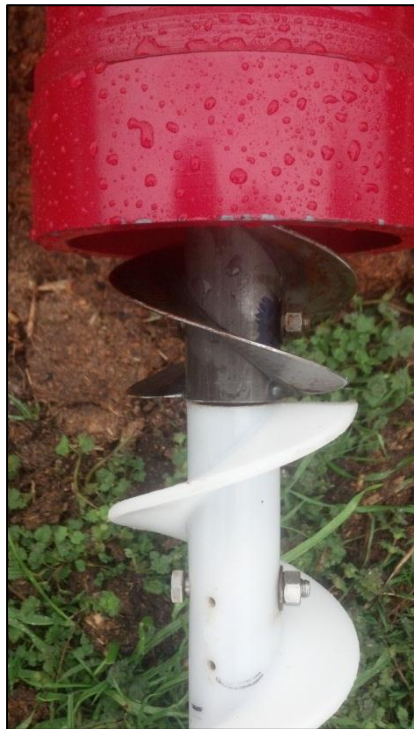
Figure 2.2 Section of double helix reverse flights connected to the HDPE single flight auger before the addition of the pipe casing.
