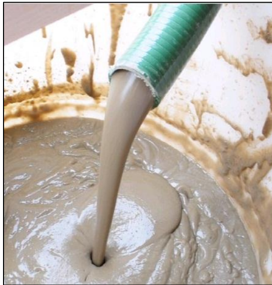
Figure B.5 Bentonite clay mixture being lifted with the Extraction Auger and recycled into a 210 L drum. Notice the material exiting the hose is less viscous than the material that is stationary in the drum due to the bentonite clay's thixotropic properties.
