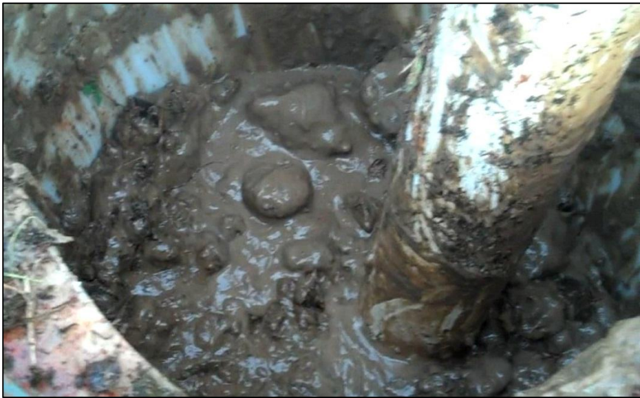
Figure C.2 7% bentonite mixture with the addition of horse manure.
