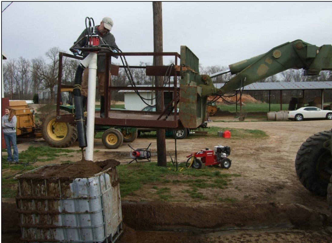
Figure C.6 Dairy farm setup to simulate emptying from a 1.8 m deep pit.
