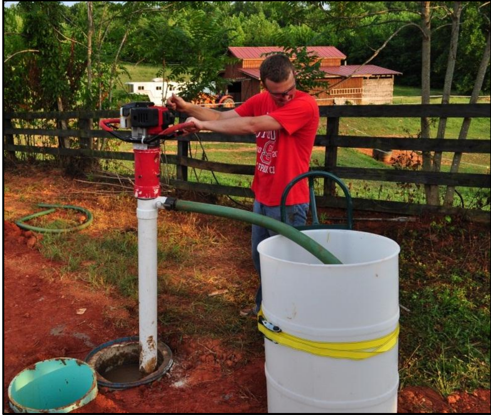
Figure 6.1 Field-testing the Extraction Auger at the Rogers farm with the 43cc 2 HP engine.
