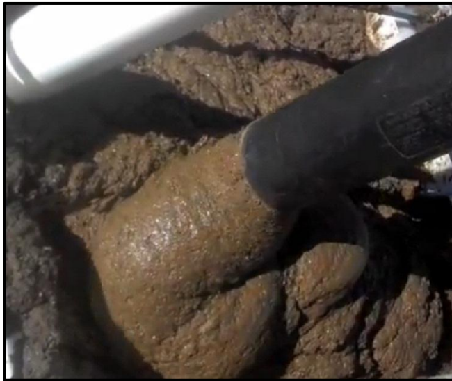
Figure 6.2 Dairy waste being recycled into the 1-m 3 container with the Hydraulic drive version of the Extraction Auger with a 2.7 m auger length.
