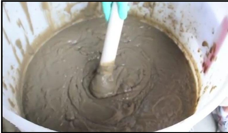
Figure B.2 7% bentonite clay mixture in a 210 L drum.
