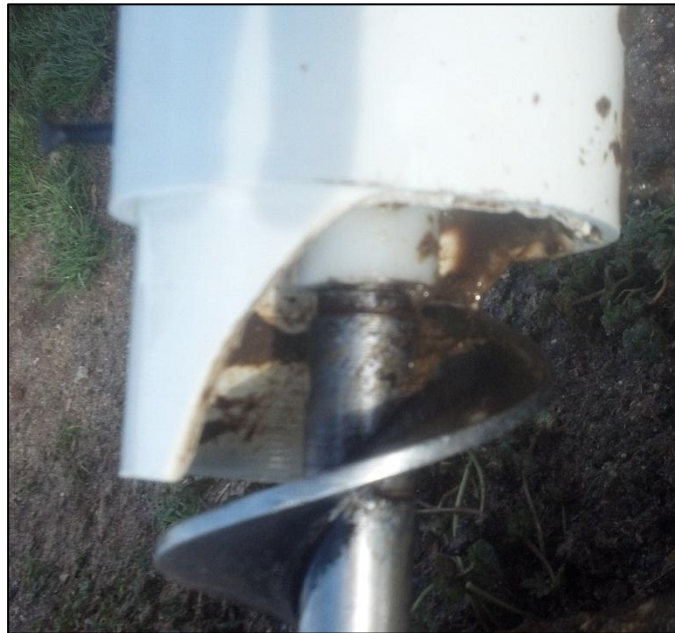
Figure C.8 The inlet of the auger after a piece was snapped off when using the hydraulic motor in the dairy waste.
