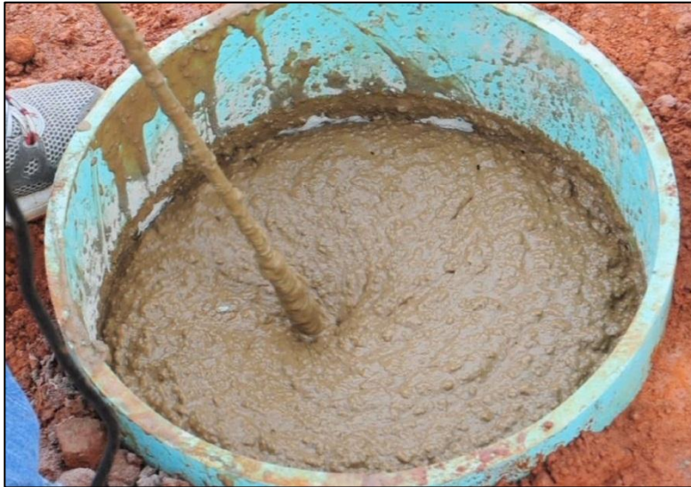
Figure C.1 10% bentonite mixture being mixed in a simulated pit.
