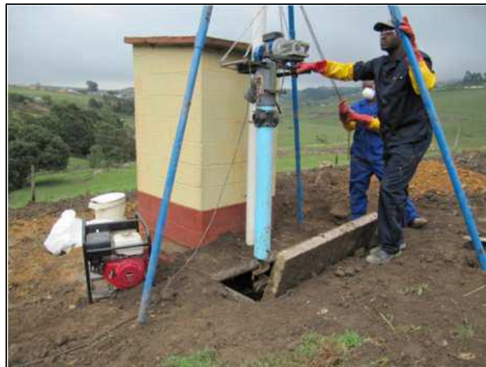
Figure A.9 Pit Screw Auger being tested in a pit latrine (Still and O’Riordan 2012).
