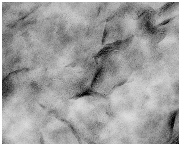
Figure 1.5: TEM image of a hectorite nanocomposite 44
