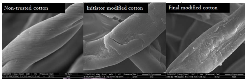
Figure 2.21. SEM of cotton fiber without treatment, initiator modified and polymer grafted. (40)
