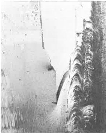
FIGURE 6: Reduction in area at the crack tip. No. 1.4948 (Type AISI 304) steel.
