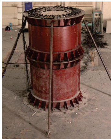
Figure 2 Test model install on base board with ceramic balls
