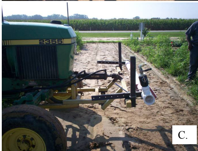
Figure 3.1. (A) Tractor-mounted Dixie wick applicator. (B) Close up of holes in PVC pipe below canvas sleeve. (C) Side view of wick with air metering orifice.
