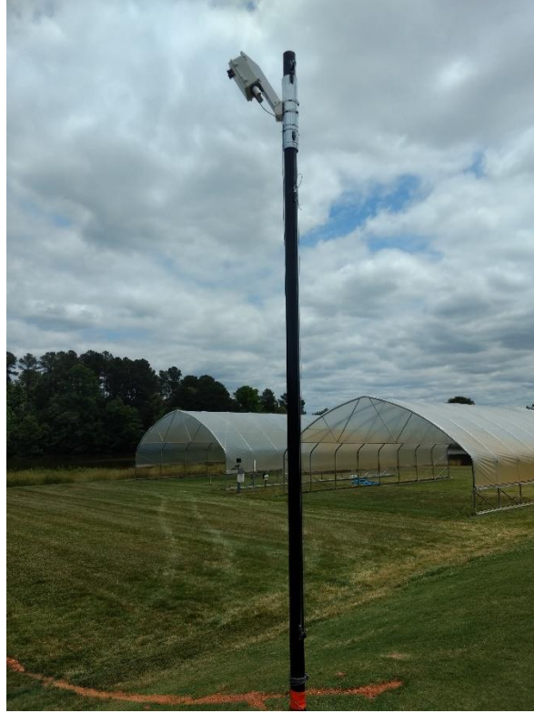
Figure 2.1: Pole Mounted camera system installed at the field site
