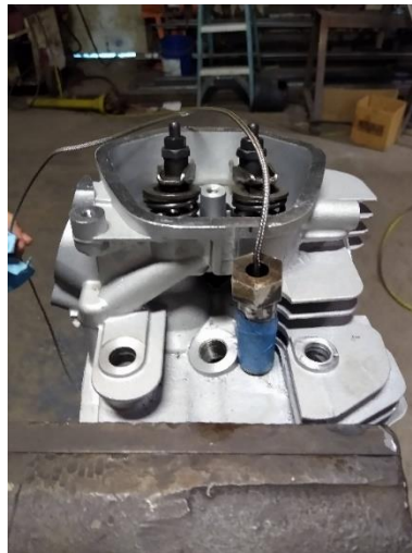
Figure 2.7: In-cylinder Pressure Sensor Installed
