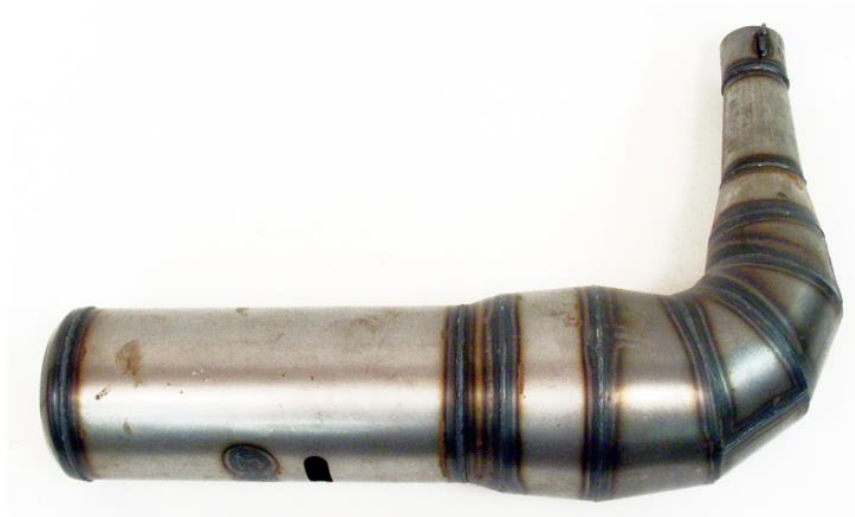
Figure 6.4: Example of a Tuned Pipe [97]
