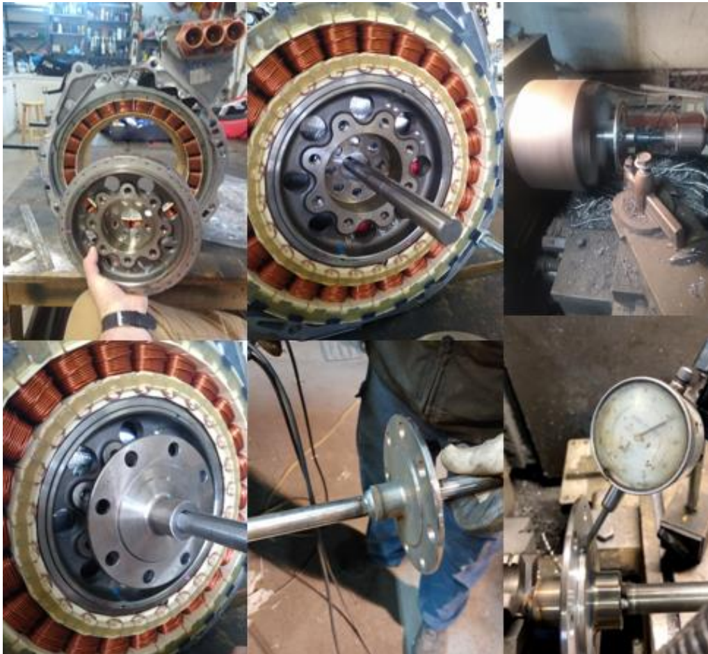
Figure 3.20: Armature Construction Collage
