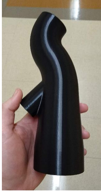
Figure 2.5: 3-D Printed Intake Runner
