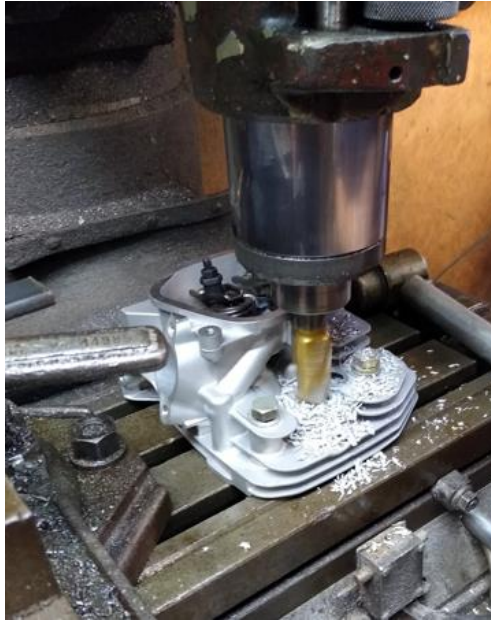
Figure 2.6: Machining the In-Cylinder Pressure Sensor
