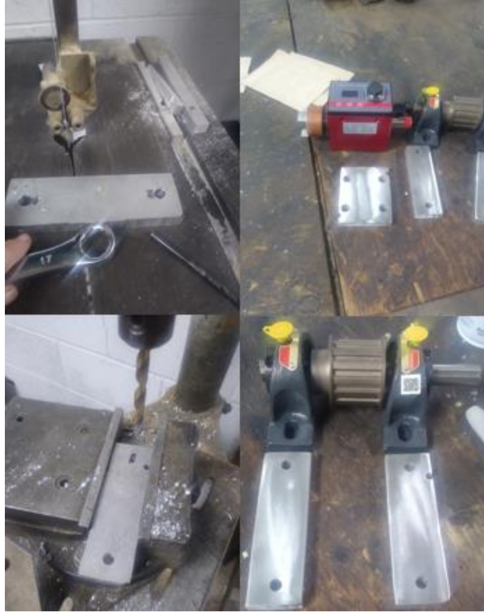
Figure 3.15: Collage of Spacer Machining
