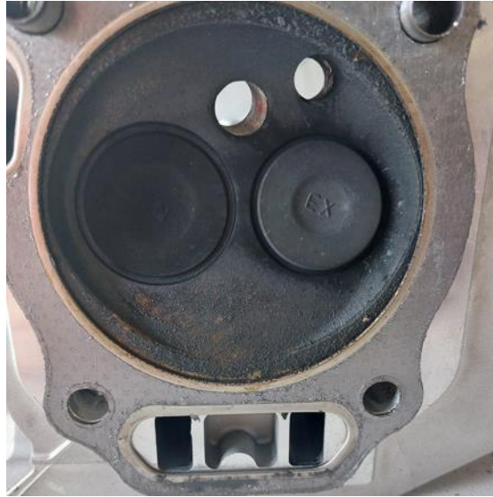
Figure 2.20: Image of Cylinder Head After Testing
