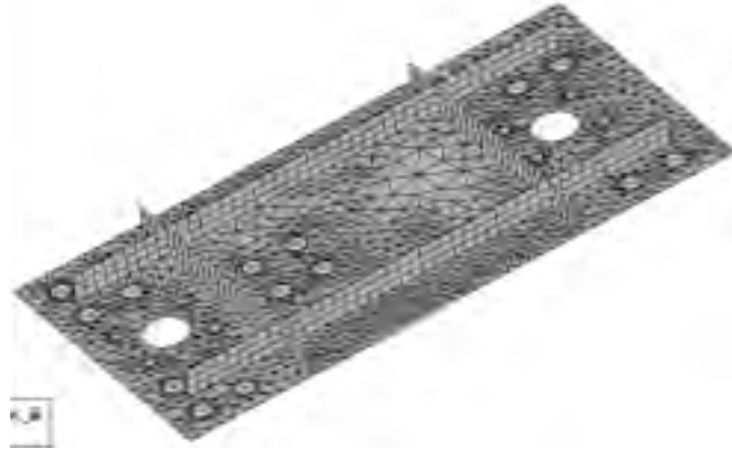
Figure 2. Typical base plate modelled with compression only springs
