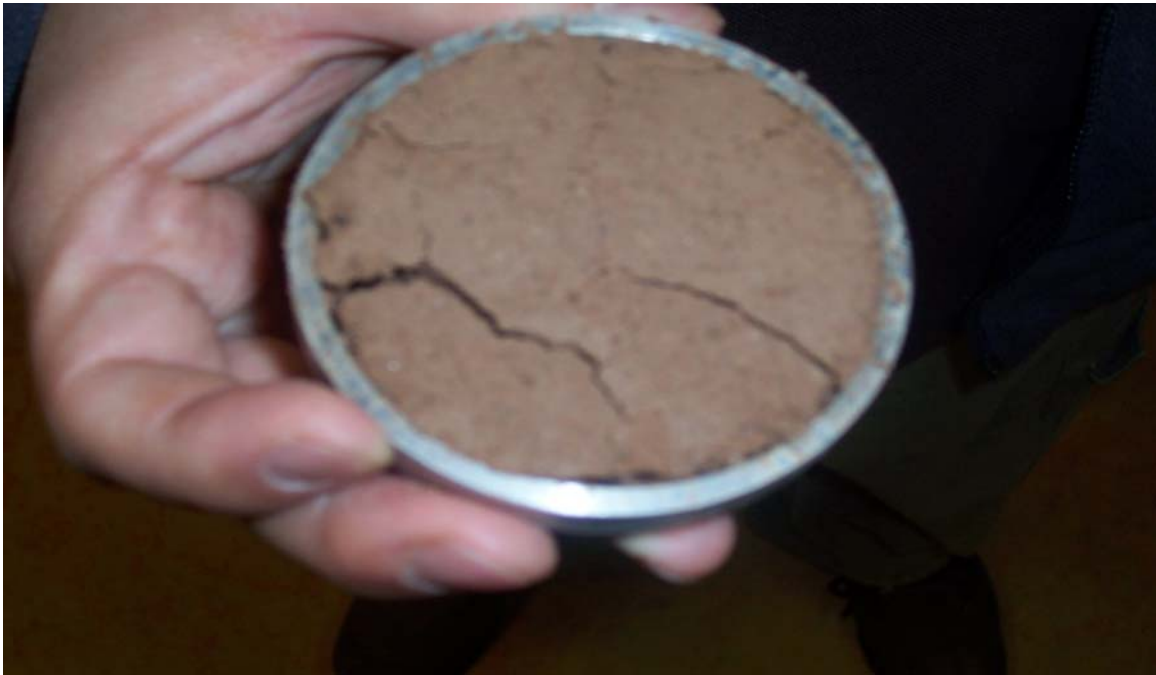
Figure 4.2.9: Pilot test low-density ( 1.51 \text{ Mg/m}^3 ) specimen (Post test-bottom view)
