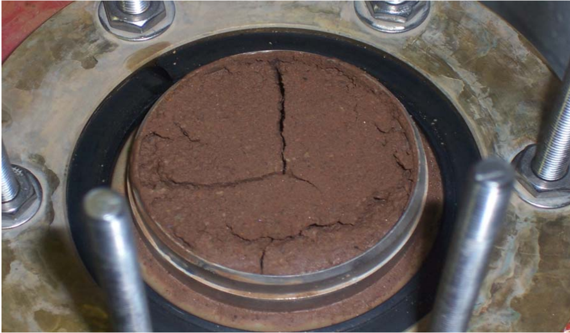
Figure 4.2.8: Pilot test low-density ( 1.51 \text{ Mg/m}^3 ) specimen (Post test-top view)
