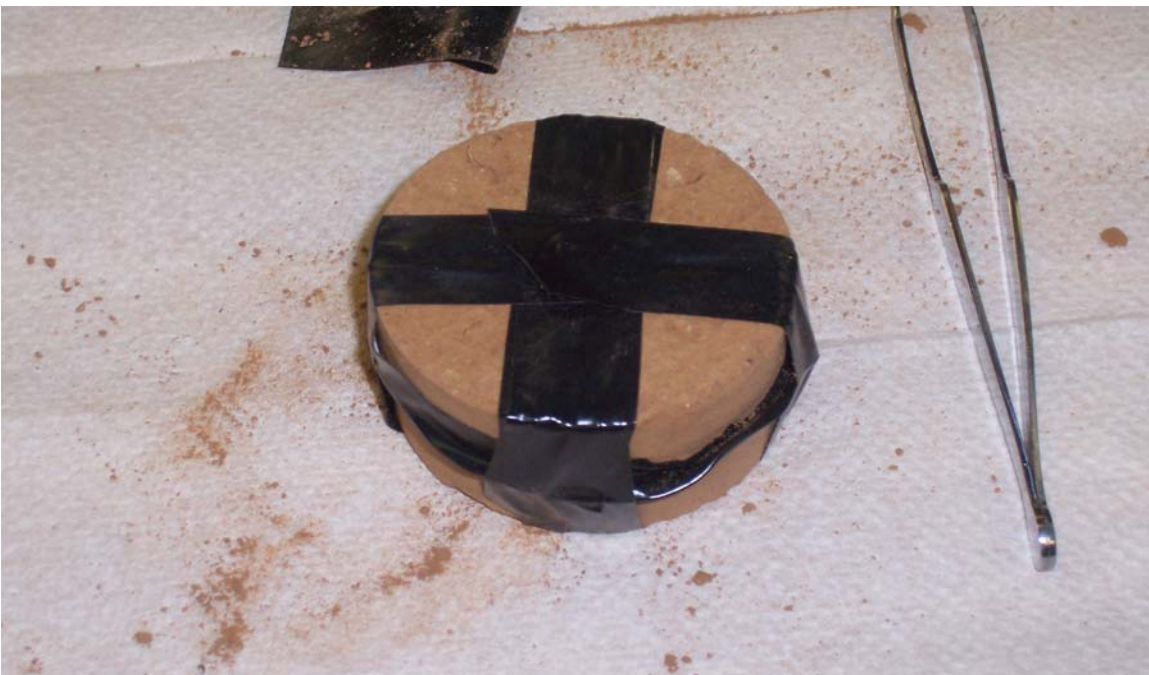
Figure 3.8.2: Compacted Material wrapped in electrical tape
