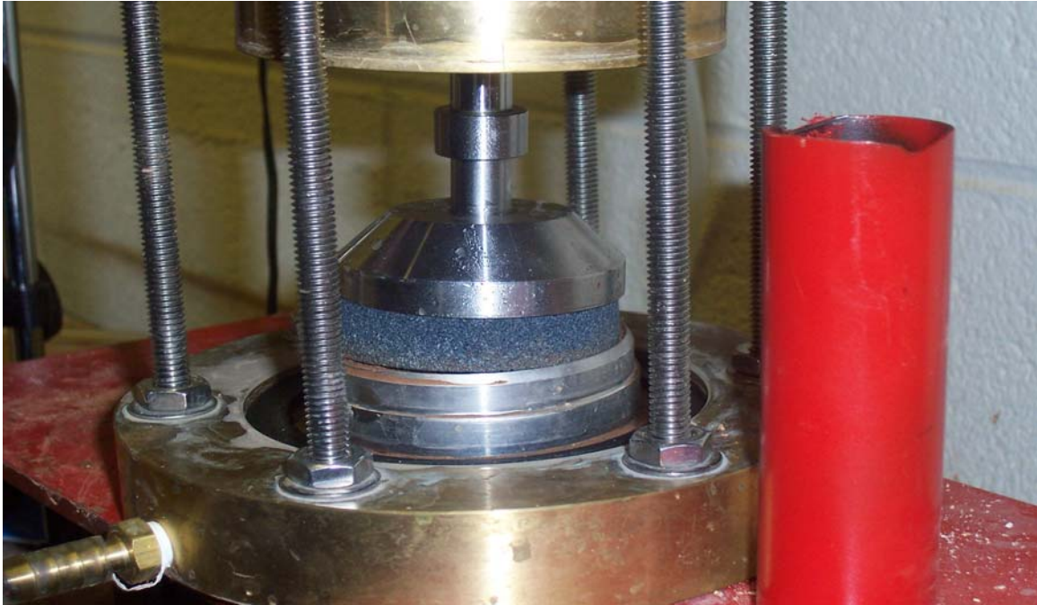
Figure 4.1.1: Compacted specimen with saturated porous stone
