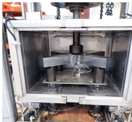
Figure 4. Five-point bending rig in the thermal chamber
