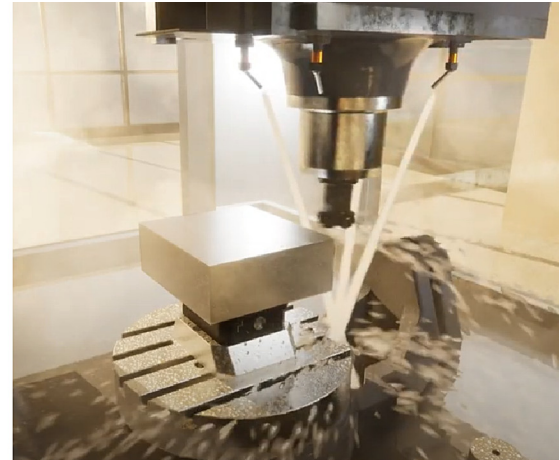
Fig. 1. A real-time simulation and visualization of a CNC cutting operation using the Unreal Game Engine 5.0 platform running on a ubiquitous nVidia RTX 3080 GPU. Coolant properties from viscosity, pressure, temperature and workpiece material properties is factored in during the simulated operation. A video playback is available at [8]
