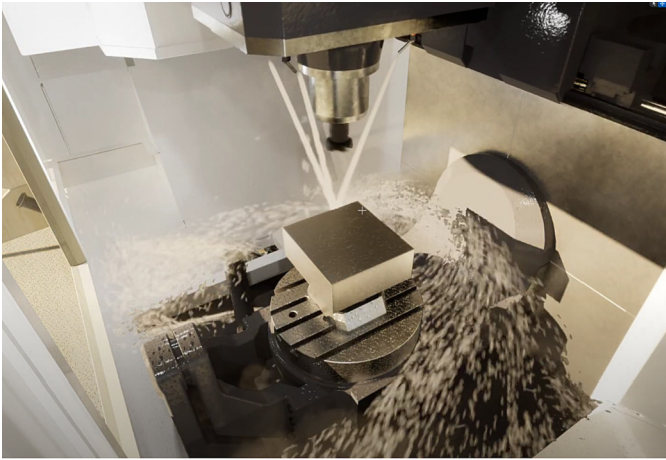
Fig. 1. A real-time simulation and visualization of a CNC cutting operation using the Unreal Game Engine 5.0 platform running on a ubiquitous nVidia RTX 3080 GPU. Coolant properties from viscosity, pressure, temperature and workpiece material properties is factored in during the simulated operation. A video playback is available at [8]
