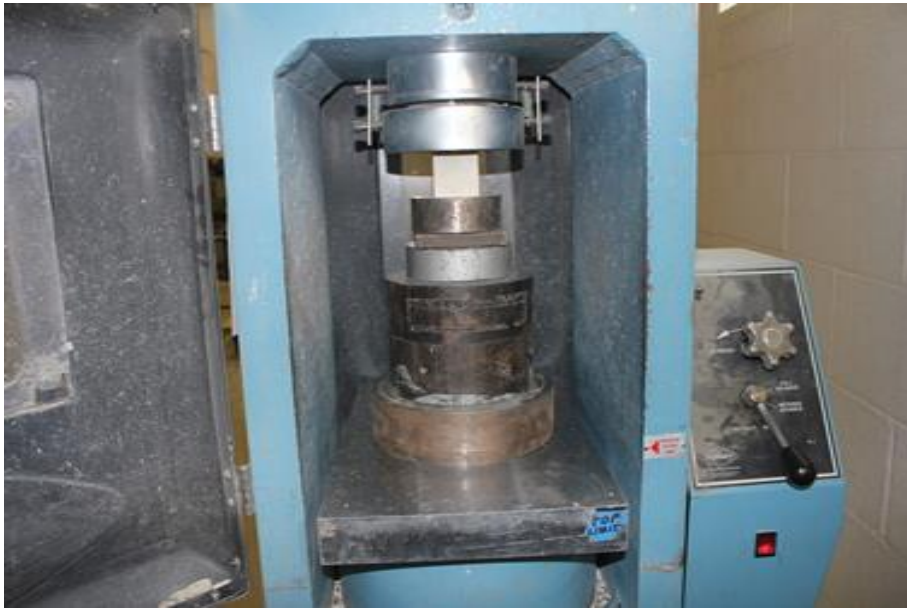
Figure 3.20 - Compressive Test Setup for Mortar Cubes
