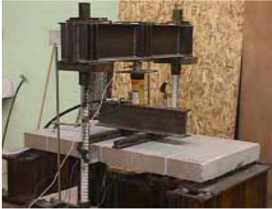
Figure 2.5 - Test Setup (Tumialan & Morbin 2002)
