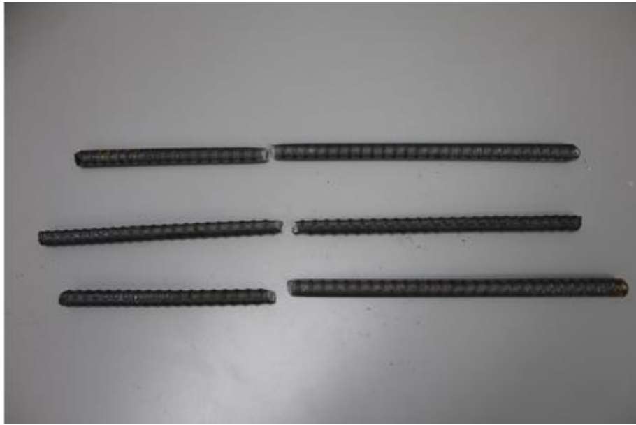
Figure 3.10 - Ruptured Steel Reinforcing Bars
