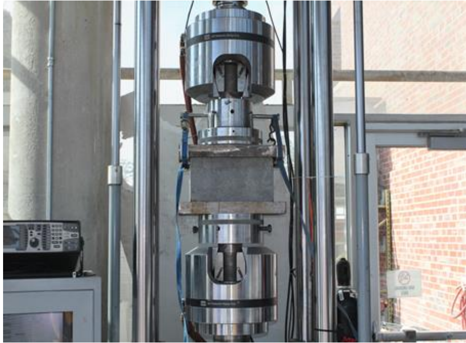
Figure 3.24 - Compressive Test Setup for Individual CMU
