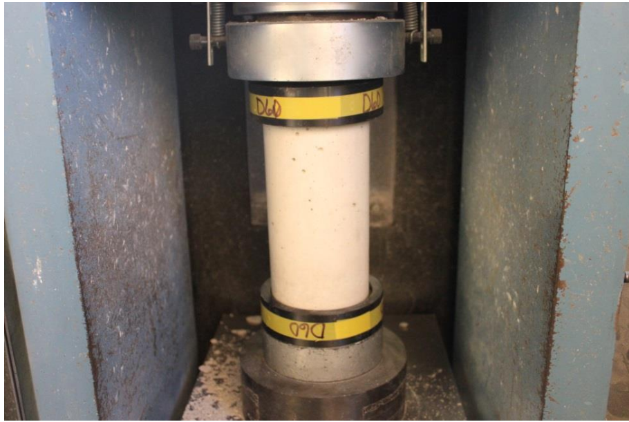
Figure 3.7 - Compressive Test Setup for Concrete Cylinders
