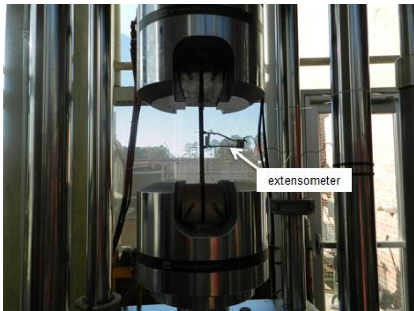
Figure 3.9 - Tension Test Setup for Steel Reinforcement
