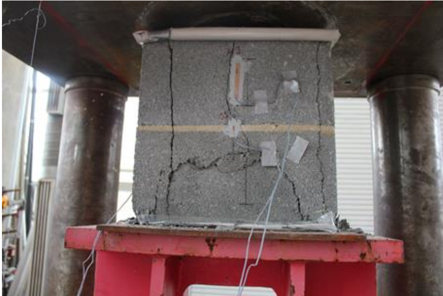
Figure 3.22 - Failed CMU Prism
