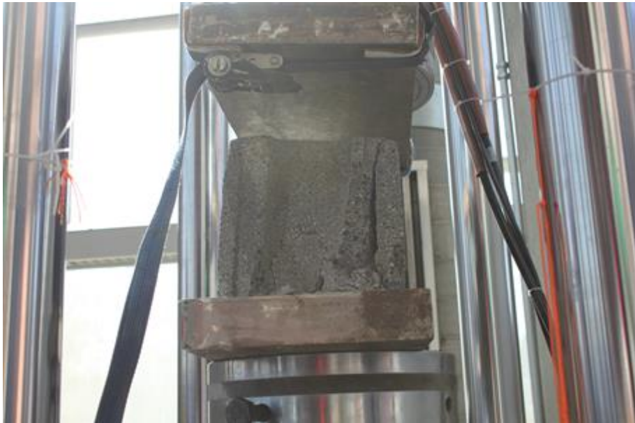
Figure 3.25 - Failed Individual CMU
