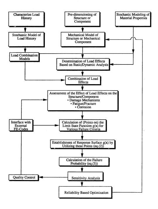
Fig. 1: COSSAN (Computational Stochastic Structural Analysis) - Schematic Flow Chart
