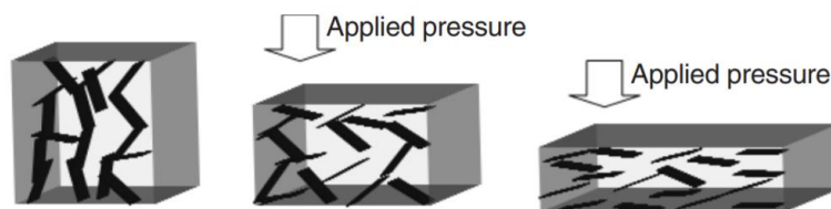
Figure 4-4 A schematic model for the change of conductive structure in the composites under pressing: the conductive fillers disperse randomly in the composite.
