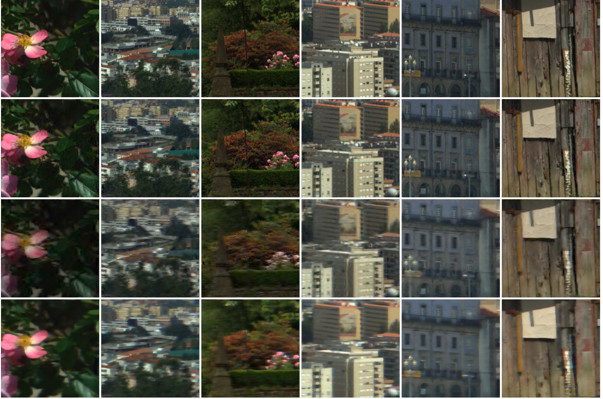
Figure 6.9: Comparison of selected image cubes reconstructed by AMP-3D-Wiener, GPSR, and TwIST for the datasets “natural scene 2002” and “natural scene 2004.” The 2D RGB images shown in this figure are converted from their corresponding 3D image cubes. Cube size is n = m = 512 , and l = 31 for images in columns 1 – 2 or L = 33 for images in columns 3 – 6. Random Gaussian noise is added to the measurements such that the SNR is 20 dB. First row: ground truth; second row: the reconstruction result by AMP-3D-Wiener; third row: the reconstruction result by GPSR; and last row: the reconstruction result by TwIST.
