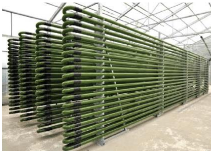
Figure 3.11: A vertical helical tubular PBR. Image reproduced from Zhang 35 .
