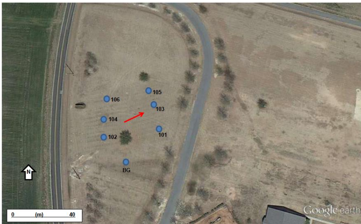
Figure 4. Piezometer locations within septic system drain field.
