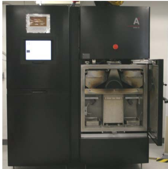
Figure 27: Photograph of an electron beam melting (EBM) machine, model A2 (Arcam AB, Mölndal, Sweden).
