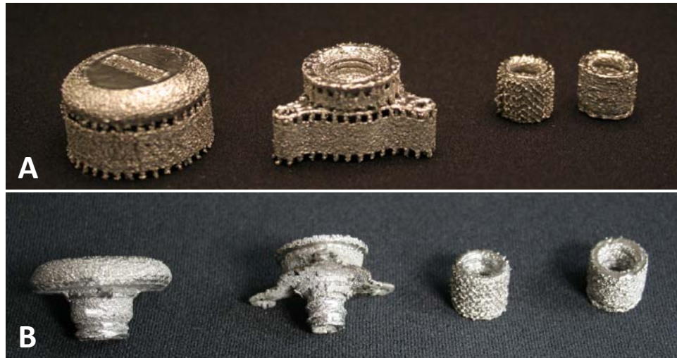
Figure 36: Transcutaneous osseointegrated implantable device components (from left to right: top cover, main body, porous threaded cap, and solid threaded cap) as fabricated with electron beam melting using Ti6Al4V powder; A) with support structure attached, B) after removal of support structure.
