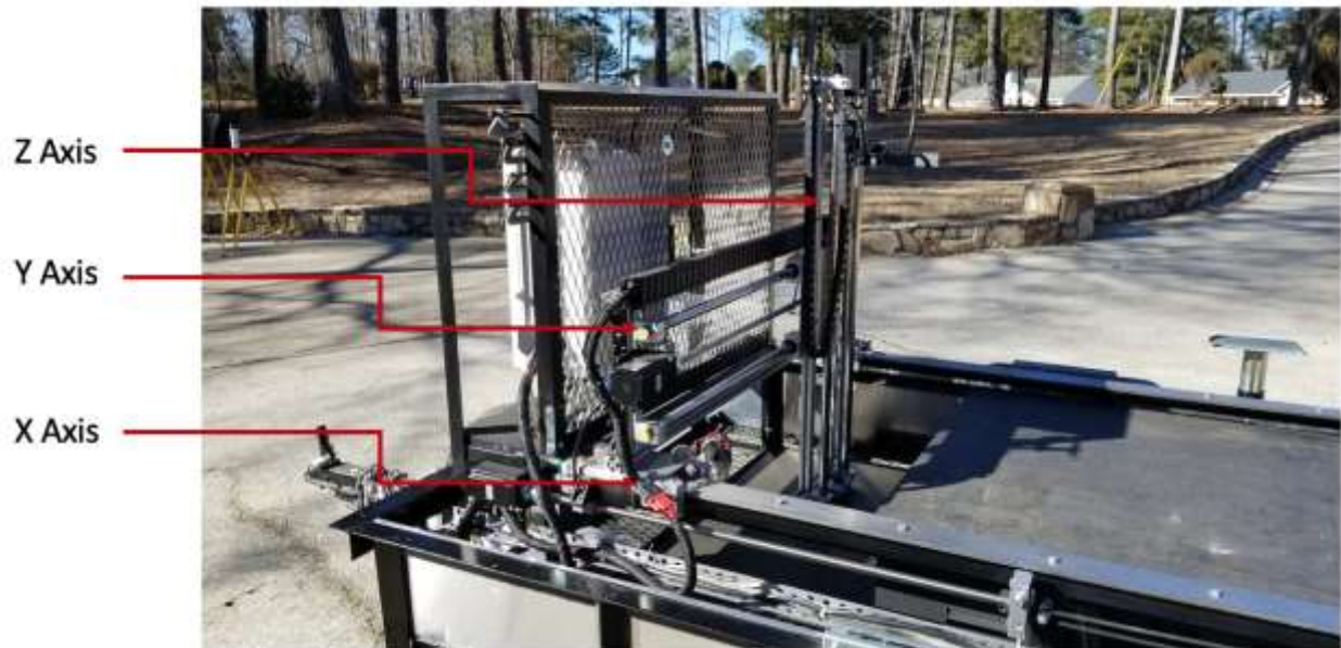
Figure 5: Battery exchange mechanism.
